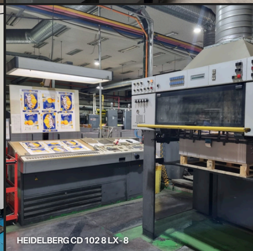
SORBUS 102-HEIDELBERG - 2 COLOR M/C CAPACITY: 10,000 SHEET/HOUR
